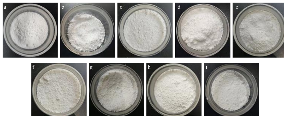
a-350FCP b-挥发油-350FCP (1:5) c-挥发油-350FCP (2:5) d-挥发油-350FCP (3:5) e-挥发油-350FCP (4:5) f-挥发油-350FCP (5:5) g-挥发油-350FCP (6:5) h-挥发油-350FCP (7:5) i-挥发油-350FCP (8:5) a-350FCP b-volatile oil-350FCP (1:5) c-volatile oil-350FCP (2:5) d-volatile oil-350FCP (3:5) e-volatile oil-350FCP (4:5) f-volatile oil-350FCP (5:5) g-volatile oil-350FCP (6:5) h-volatile oil-350FCP (7:5) i-volatile oil-350FCP (8:5)
